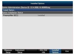
If the correct key code is entered, the R&S FSC displays "Installation successfull", and the option is marked as "Installed" in the option list (example: Option Preamplifier (B22)).
