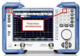
7. Switch the instrument on and keep PRESET and '8' pressed for at least 5 seconds after the startup screen has appeared on the screen.
